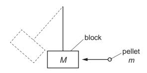
A pellet of mass m travelling at a speed u hits a stationary block of mass M. The pellet becomes embedded in the block and causes the block to move at a speed v immediately after the impact.
